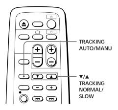
you press one of the two buttons. If you cannot get a clear picture with manual adjustment, press TRACKING AUTO/MANU to return to automatic adjustment.
